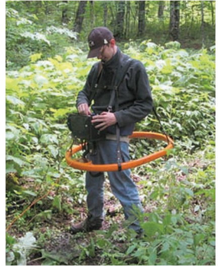
Joshua Shue sets the frequency on the horizontal loop transmitter during an electromagnetic survey near Taylor Mine. Students used electromagnetic techniques to detect and map the location of conductive slates.
