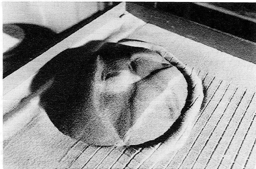
Figure 3. Oblique view of a spreading analogue volcano (Figures 3a, 3b, and 3c are experiment 3 with \Pi_2=0.3 , \Pi_3=1.1 , \Pi_4=1 ; width of the box is 50 cm). (a) Initial stage. (b) Smoothed relief due to the spreading process 2 hours after figure 3a. (c) Upper free surface at the end of the experiment (10 hours) showing four grabens in the analogue volcano and a concentric thrust zone around it. Displacements occurred in unbuttressed directions only. This pattern is remarkably similar to the one observed at Etna volcano (Figure 5).
