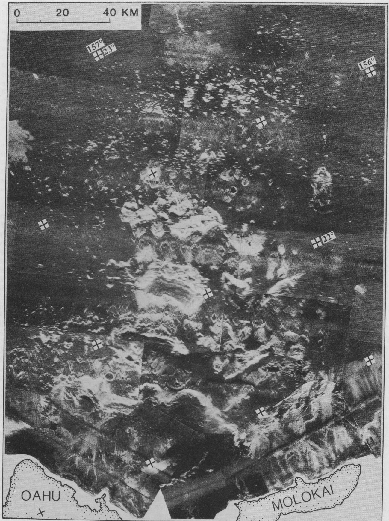
Fig. 7. Mosaic of GLORIA sonographs showing the Nuuanu and Wailau debris avalanches. Light shades designate regions of greater acoustic backscatter. The apparent elongation of hummocks parallel to ship tracks is an artifact caused by yaw of the towed vehicle.
