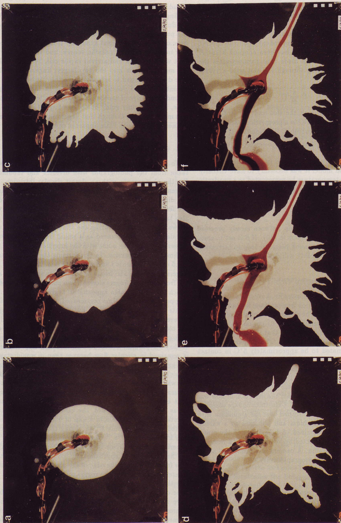
Plate 1. Photographs of the evolution of paraffin flowing with constant volume flux through a cooled slot from a point source. From left to right: (a) At 12 s after start of the experiment a circular intrusion is seen. (b) At 16 s two small notches have grown. (c) By 20 s numerous fingers break out. (d) At 24 s the fingers have grown considerably. (e) At 52 s, dye reveals there is flow through two channels; there is also evidence that third channel stopped just as the dye entered the tank. (f) At 92 s, darker dye reveals that there is flow in only one channel.
