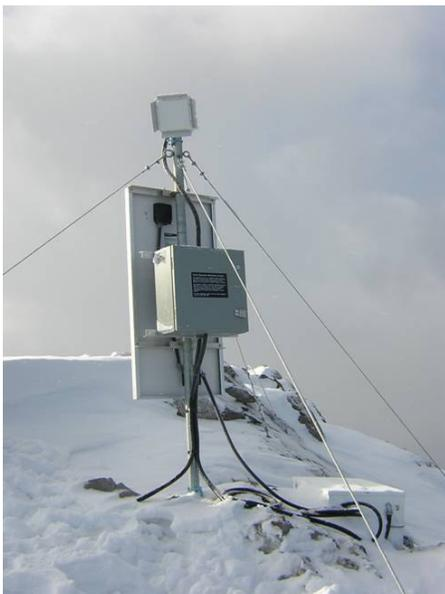
Figure 8. Typical surface seismic station installed on South Peak of Turtle Mountain.
