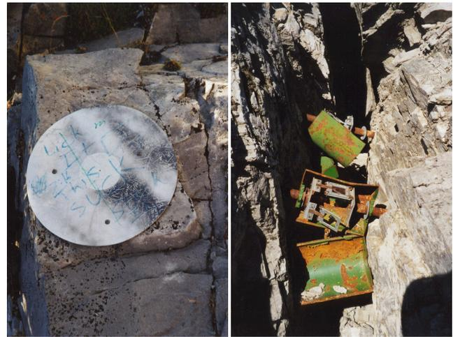
Figure 7: Defaced photogrammetry target (left) and vandalized Moiré crack gauges (right) observed in 1999.
