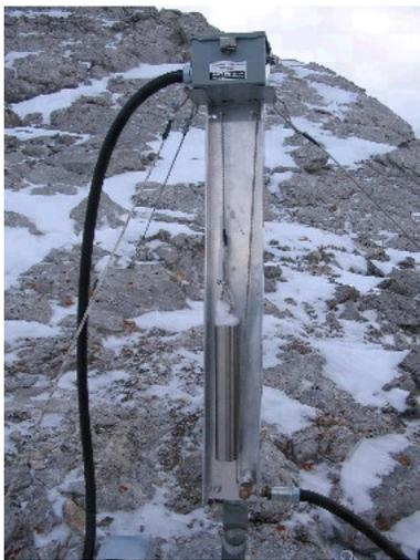
Figure 12. Typical surface extensometer head assembly with housing removed to show suspended weight.
