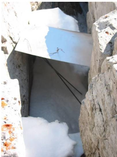
Figure 10. Vibrating wire crackmeters installed across a major fissure. The metal snow roof is to protect the instruments.
