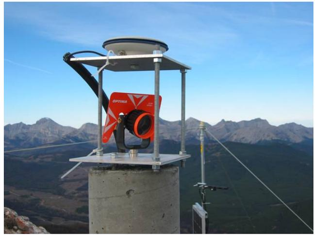
Figure 11. Combination theodolite prism and GPS antenna mounted on a concrete pillar near South Peak.
