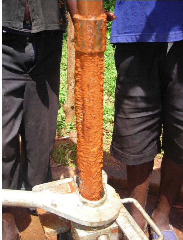
Figure 1.2 Orange slime found on galvanized iron riser pipes extracted from the well in Bulegete (photograph by author)
