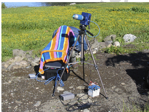
Fig. 1. Field set-up of UV camera and associated components. The camera and lens are mounted on a tripod, and connected to the laptop computer (kept under the towel, due to glare). The laptop and camera are powered by two 6-volt batteries, although other power sources are possible.
