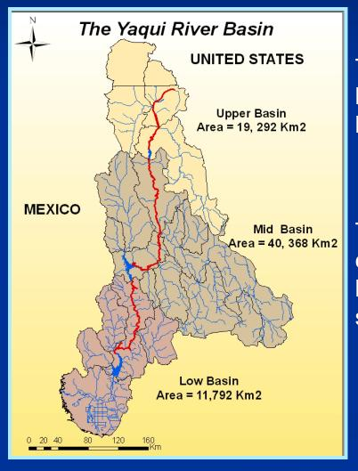
The watershed and sub-basin boundaries were delineated using GIS based on DEMs.
