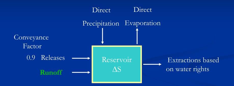
$\Delta S_{i} = \Delta S_{i-1} + \text{Rumoff} + \text{Precipitation} + 0.9 \text{ Releases} - \text{Evaporation} - \text{Extractions}$  $\frac{\text{RUNOFF}}{\text{RUNOFF}} = Y_{ij}$
