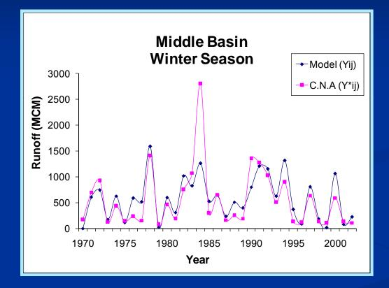
The timing of the peaks matches reasonably well, but the model tends to under predict the runoff in the wettest year (1984).
