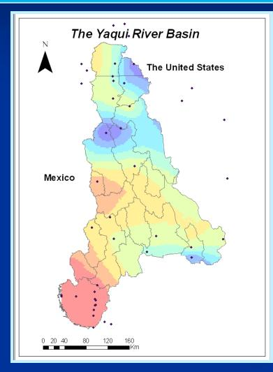
Precipitation data was interpolated on a monthly basis over a 33-year time span using GIS.
