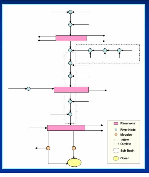
A node- link network is the conceptual basis for the model.
